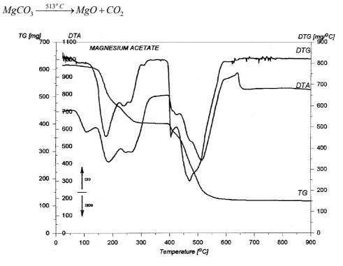
Fig. 4. Thermal decomposition of magnesium acetate
