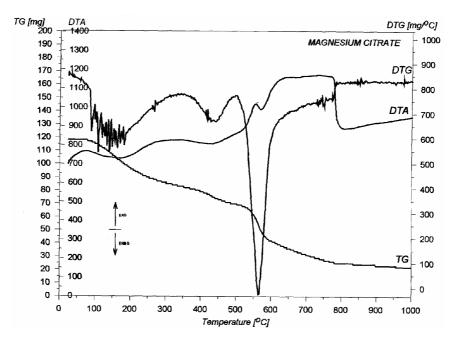
Fig. 5. Thermal decomposition of magnesium citrate
