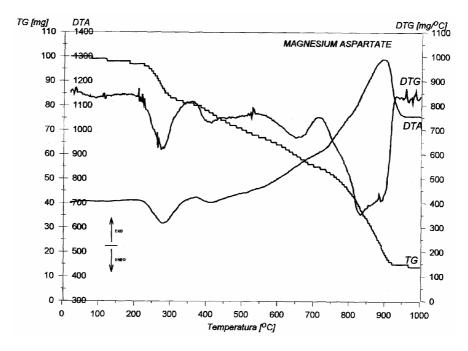
Fig. 6. Thermal decomposition of magnesium asparate
