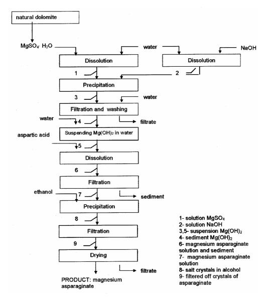
Fig. 3. Scheme of preparation of magnesium asparaginate
