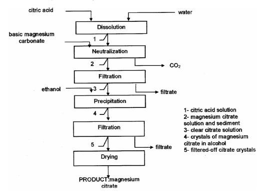
Fig. 1. Scheme of preparation of magnesium citrate
